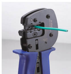
Press gradually and crimping well
